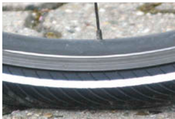
Figure 90: Correct tyre pressure. The tyre is barely deformed under the load of the body weight.
