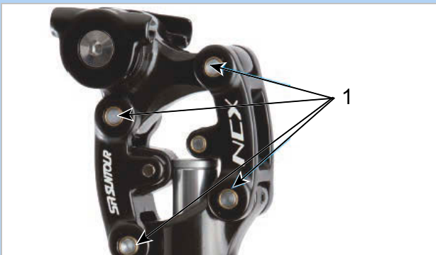
Figure 187: SR SUNTOUR suspension seat post lubrication points
