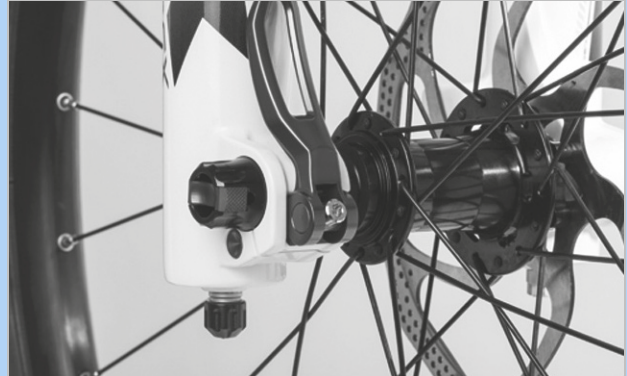
Figure 185: Adjusting the quick release clamping force
