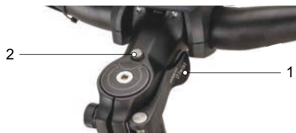
Figure 63: Stem, version II with clamping lever on the stem quick release (1) and unlocking knob (2)
