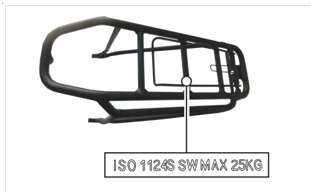
Figure 130: The maximum load bearing (1) capacity is indicated on the pannier rack
