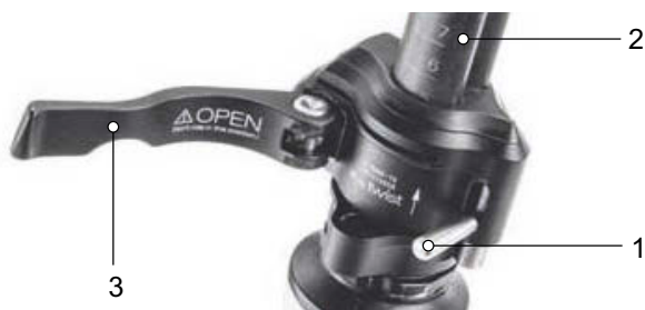
Figure 62: Opened clamping lever on the stem quick release (3) on the stem (2), version I, with locking lever on the stem (1)
