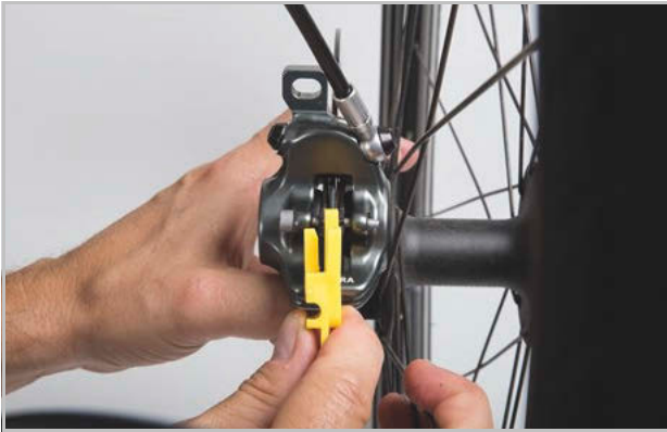
Figure 157: Checking the brake lining when fitted with the help of the transport safety wear gauge
