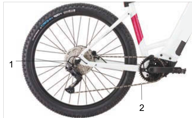
Figure 33: Chain drive with derailleur gears
