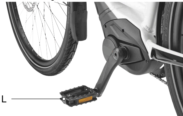
Figure 65: L pedal in the left-hand crank arm
