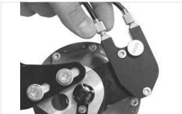
Figure 182: The tension adjuster on ROHLOFF hub versions with external switch control is located on the cable box positioned on the left-hand side
