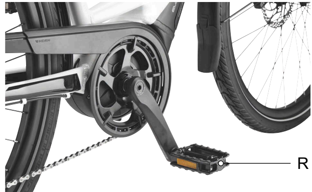
Figure 66: R pedal in the right-hand crank arm
