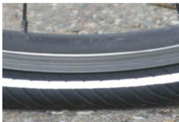
Illustration 109 : Pression largement insuffisante
