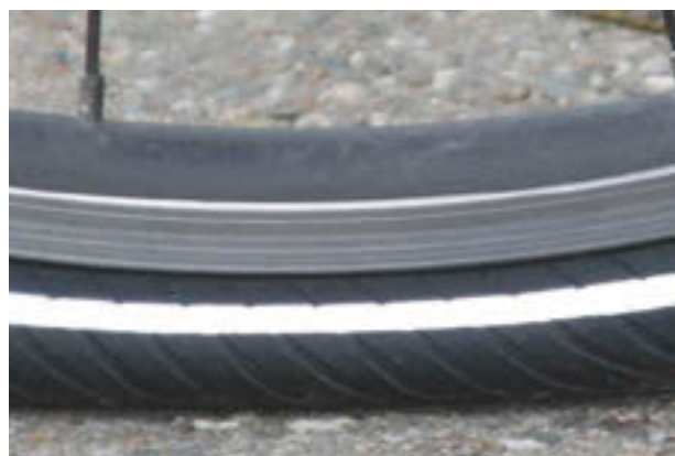
Illustration 86 : Pression largement insuffisante
