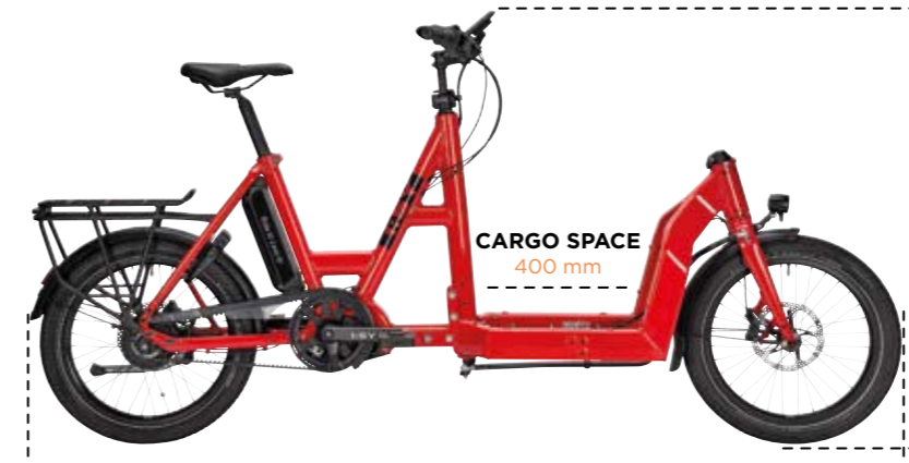
i:SY CARGO OVERALL LENGTH 2.130 mm (Mod. 23) | 2.180 mm (Mod. 24)
