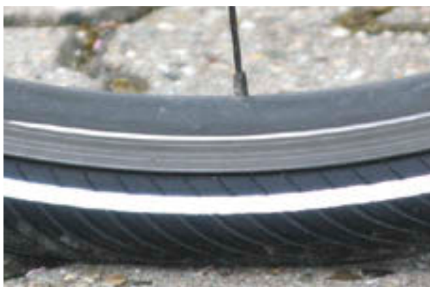
Figure 96: Correct tyre pressure. The tyre is barely deformed under the load of the body weight
