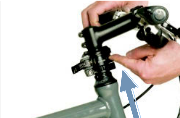
Figure 172: Pressing the unlocking bolt upwards
