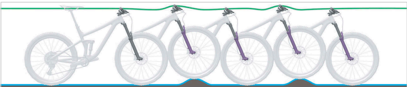
Figure 17: Optimum suspension fork ride performance
