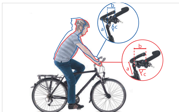
Figure 94: City bike (blue) and trekking bike position (red) by changing the angle
