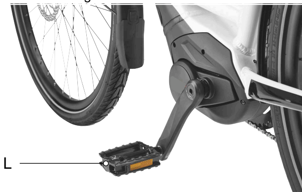
Figure 79: L pedal in the left-hand crank arm
