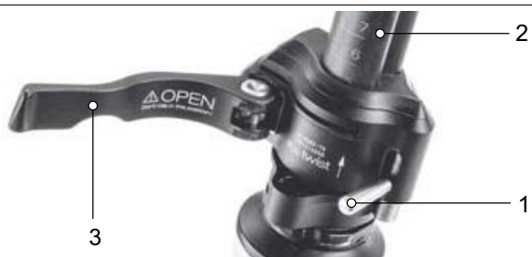
Figure 76: Opened clamping lever on the stem quick release (3) on the stem (2), version I, with locking lever on the stem (1)
