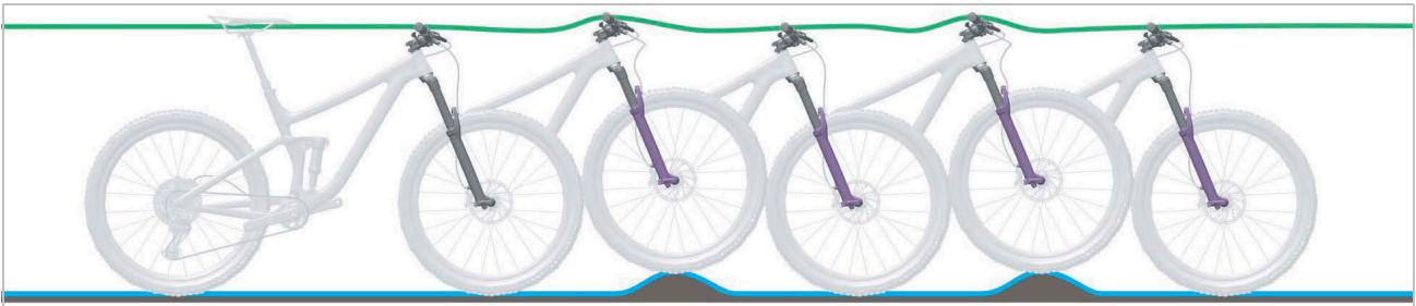
Figure 14: Optimum suspension fork ride performance
