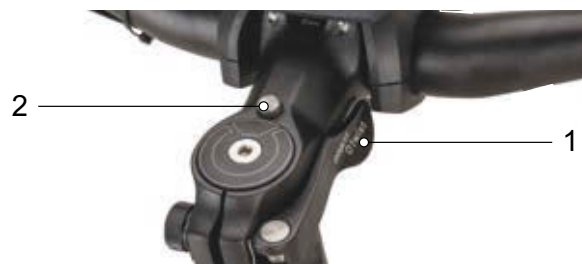
Figure 77: Stem, version II with clamping lever on the stem quick release (1) and unlocking knob (2)
