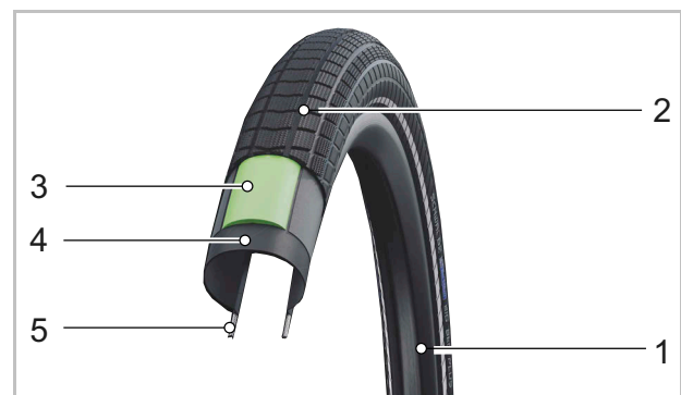
Figure 25: Structure of tube-type tyres
