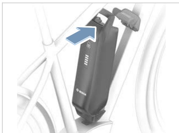
Figur 155: PowerPack-batteriet klappes opad
