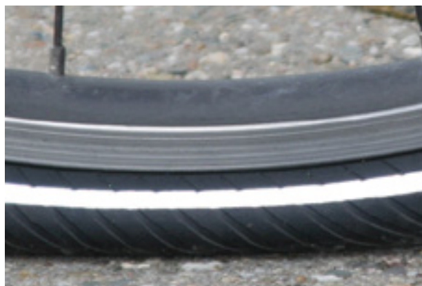
Illustration 68 : Pression largement insuffisante
