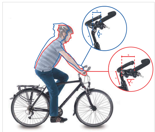
Figure 92: City bike (blue) and trekking bike position (red) by changing the angle
