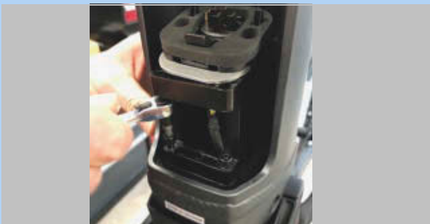
Figure 53: Removing the 4 mm hexagon screws
