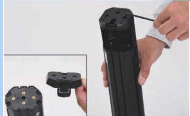
Figure 63: Fastening the battery mounting plate
