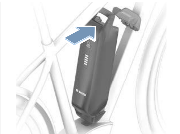
Figure 136: Closing the PowerPack battery upwards
