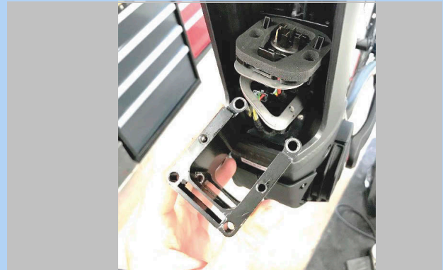
Figure 55: Pulling out the PowerTube adapter
