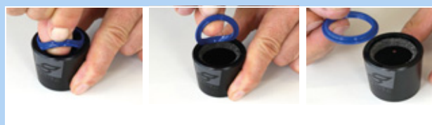
Illustration 127 : Retirer le joint anti-poussière
