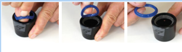
Illustration 162 : Retirer le joint anti-poussière
